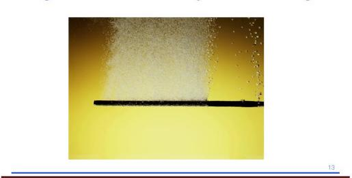
Figure 19: Pore Size Measured by Bubble Point Testing
